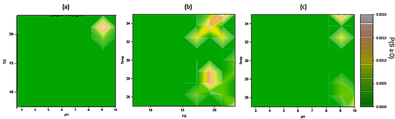
**Fig. 3.** Probability surfaces to reach  $S \geq 0$ : (a) pH versus TG (min.), (b) TG (min.) versus  $T^\circ$  ( $^{\circ}$ C), (c) pH versus  $T^\circ$  ( $^{\circ}$ C).
