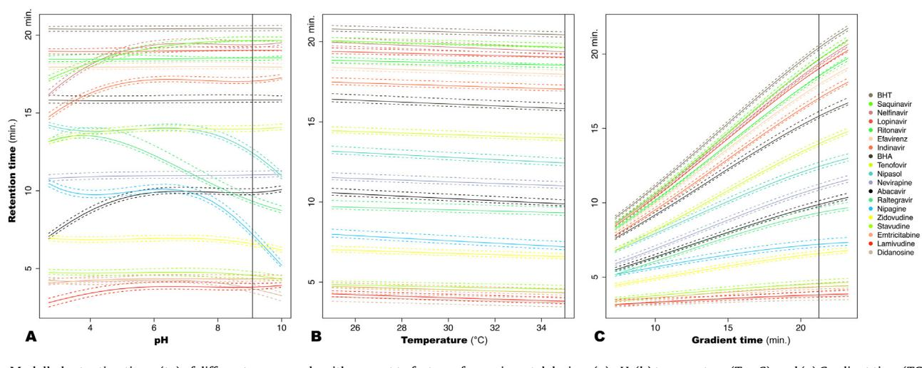
**Fig. 2.** Modelled retention times ( $t_R$ ) of different compounds with respect to factors of experimental design: (a) pH, (b) temperature ( $T^\circ$ , °C), and (c) Gradient time (TG, min).
