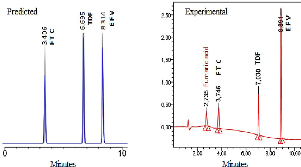
**Fig. 9.** Predicted and experimental chromatograms of FTC/TDF/EFV combination. Resolutions are 6 (between Fumarate and FT), 27 (between FTC and TDF) and 24 (between TDF and EFV).
