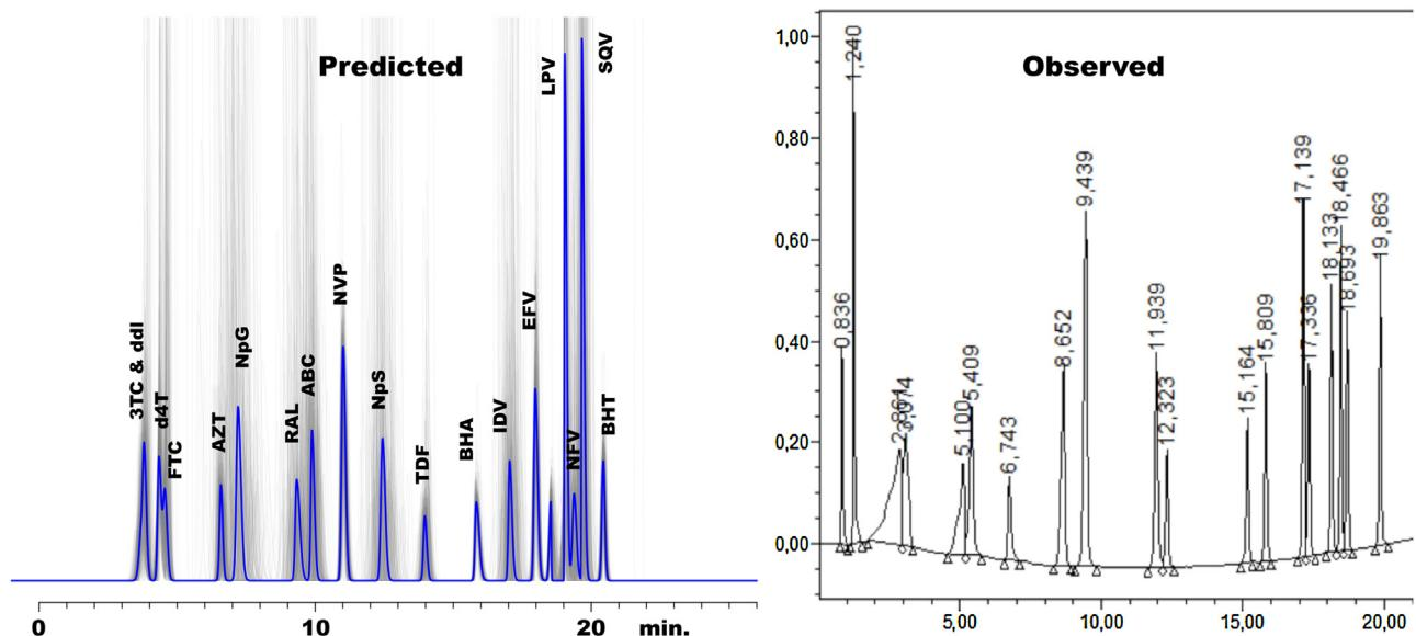
**Fig. 4.** (a) Predicted chromatogram for the screening method. (b) Experimental chromatogram for the screening method on the overall solution.
