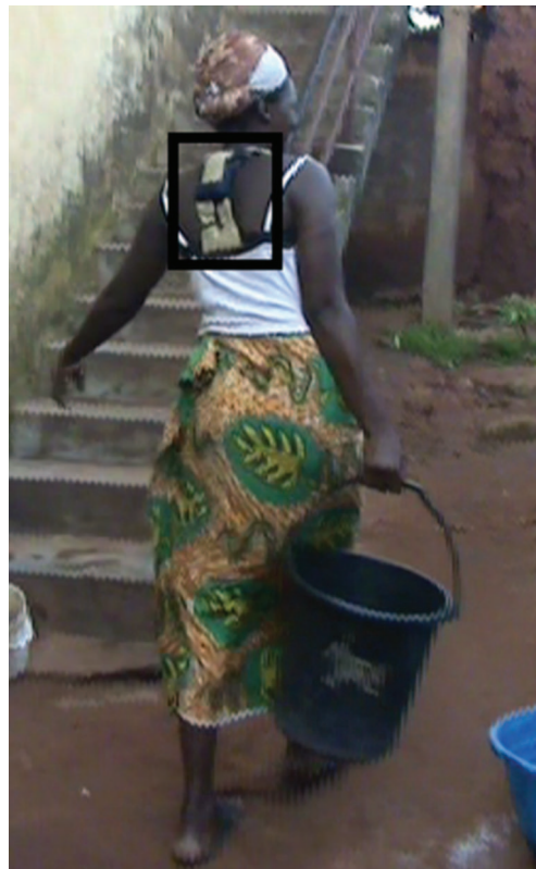
Figure 1. Pregnant women instrumented with one VC at the level of C7. The VC is enclosed in the navy blue pocket to minimise its displacement (shown in black box). Tape was also used over the adjustable feature of the harness to secure it to the women's torso.
