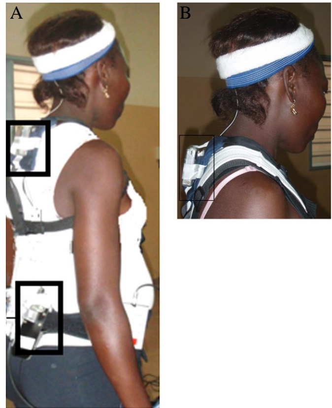
Fig. 1. A) The two VCs worn by a pregnant woman at C7 and sacrum levels. The VC at C7 is secured in a small custom pocket attached to the subject around the torso and shoulders. The VC at sacrum is attached to a belt fastened around the waist. B) Zoomed view of picture (A) to show the electrogoniometer attached by the headbands and a close view of the VC at C7.
