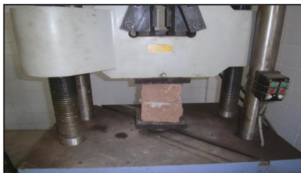
Figure B compressive strength test on CEB
