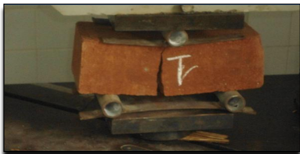
Figure A flexural strength test three points on BT
